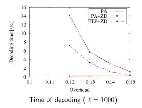
We can reduce the latency of decoding
