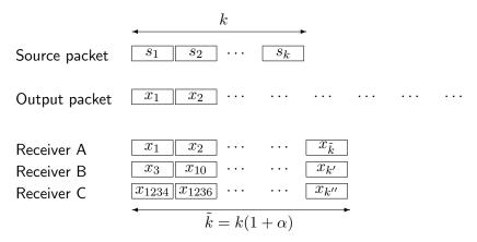
Even if packet losses occur, receiver can recover source packets
